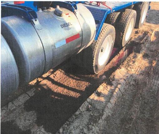
**Truck fuel tank leaked Diesel**
