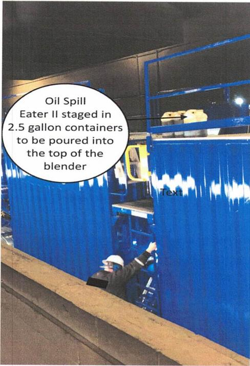
Oil Spill Eater II is poured into the top of the blender, and once OSE II has circulated for a short time the blender is drained directly into floor drains in the shop. The drain is also kept clean with the OSE II in the effluent from the blender as well
